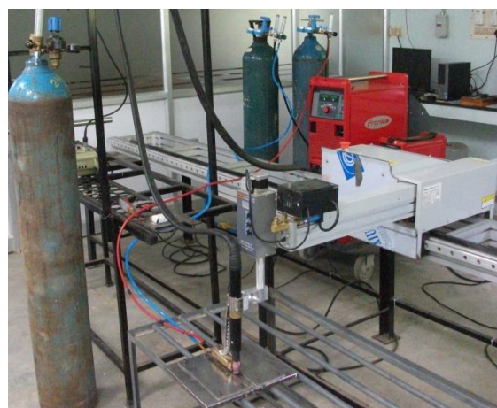
Figure 1 Automated TIG welding setup
